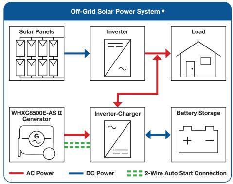
♦ Depending upon system configuration, the generator can automatically provide backup to recharge the storage battery and / or feed in power to supply the load.
